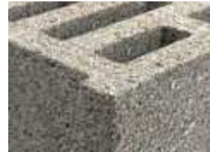
Hollow blocks made from concrete
