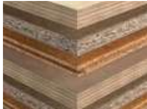
Wooden boards (e.g. OSB, chipboard, MDF and plywood boards)
